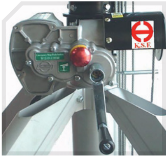
Manual use With crank provided
